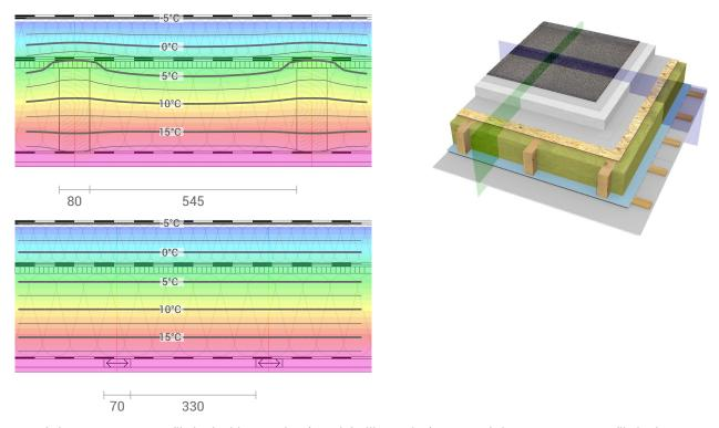
Top left: Temperature profile in the blue section (see right illustration). Bottom left: Temperature profile in the green section.
