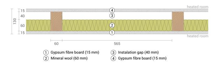
Inside air :  $20,0^{\circ}$ C / 50% Thickness: 13,0 cm Inside air 2:  $20,0^{\circ}$ C / 50% sd-value: 0,5 m Weight: 40 kg/m² Surface temperature.:  $20,0^{\circ}$ C /  $20,0^{\circ}$ C Heat capacity: 47 kJ/m²K
