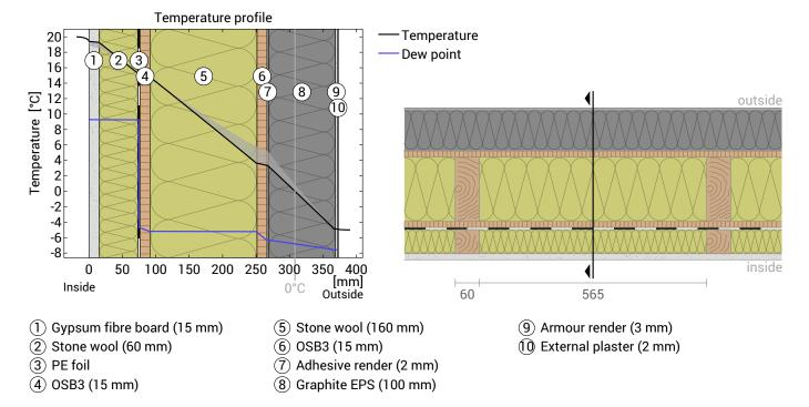
**Left:**Temperature and dew-point temperature at the place marked in the right figure. The dew-point indicates the temperature, at which water vapour condensates. As long as the temperature of the component is everywhere above the dew point, no condensation occurs. If the curves have contact, condensation occurs at the corresponding position. **Right:** The component, drawn to scale.
