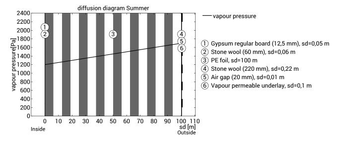
Condensate-free component: The maximum possible evaporation mass for the drying reserve is calculated. Consider the level that has the lowest evaporation potential in the dew period, at sd=100,34 m; x=31,27 cm:
