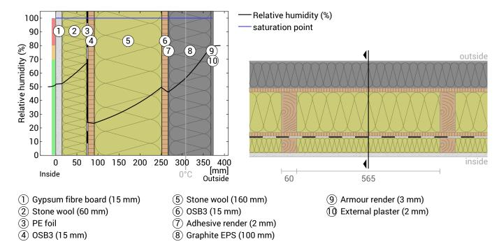
Notes: Calculation using the Ubakus 2D-FE method. Convection and the capillarity of the building materials were not considered. The drying time may take longer under unfavorable conditions (shading, damp / cool summers) than calculated here.
