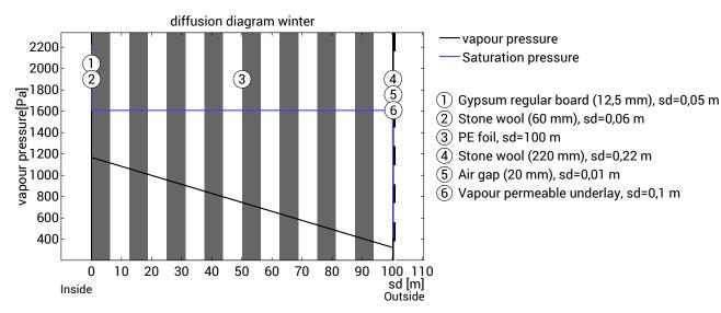
The section under investigation is free of condensate under the given climate conditions.
